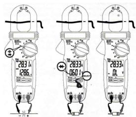
**Note**: When using diode test function, normal forward voltage drop (forward biased) for a good silicon diode is between 0.400V to 0.900V. A reading higher than that indicates a leaky diode (defective). A zero reading indicates a shorted diode (defective). An OL indicates an open diode (defective). Reverse the test leads connections (reverse biased) across the diode. The digital display shows OL if the diode is good. Any other readings indicate the diode is resistive or shorted (defective).
