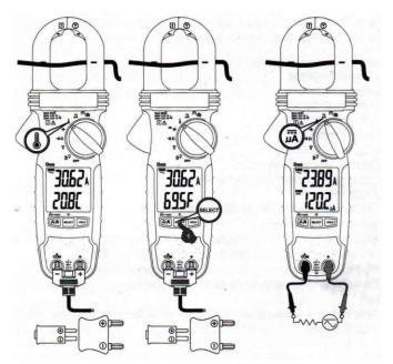
**Note**: Be sure to insert the banana plug type-K temperature bead probe Bkp60 with correct + - polarities. You can also use a plug adapter Bkb32 (Optional purchase) with banana pins to type-K socket to adapt other type-K standard mini plug temperature probes.
